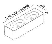
Note: It is available with a minimum length of 128,2 cm and a maximum length of 240 cm. L\* = nominal size, real length - 26 mm
