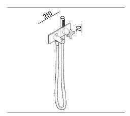
Built-in single lever tap unit with gradual flow control with flow deviator and handheld shower holder. Finished items to complete with shower heads, flexible hoses and handheld showers.
