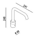
Countertop washbasin spout with electronic sensor, equipped with external solenoid valve for water mixing (6V power supply included)
